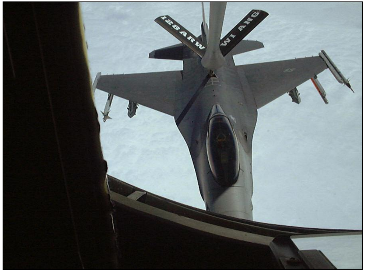
An F-16 is refueled through a boom in mid-air by a KC-135. The F-16 is about 35 feet from the refueling plane. The KC-135 flies at 530 miles per hour at 30,000 feet and can take off with a gross weight of up to 322,500 lbs. Several planes were refueled enroute from Milwaukee to Norfolk, Virginia.
